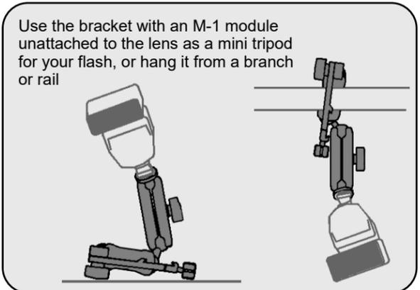
Use the bracket with an M-1 module unattached to the lens as a mini tripod for your flash, or hang it from a branch or rail
