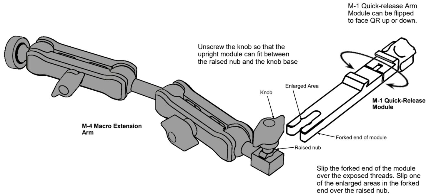
Unscrew the knob so that the upright module can fit between the raised nub and the knob base
