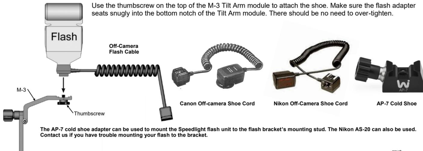
The AP-7 cold shoe adapter can be used to mount the Speedlight flash unit to the flash bracket's mounting stud. The Nikon AS-20 can also be used. Contact us if you have trouble mounting your flash to the bracket.
