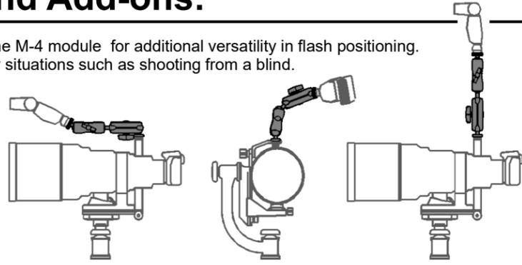
**Macro Flash Bracket (F-2):** The Macro Arm (M-4) can also be used to connect directly to the Quick-Release Arm (M-1). This is commonly used in macro applications or with small cameras and lenses where the upright module is not necessary.
