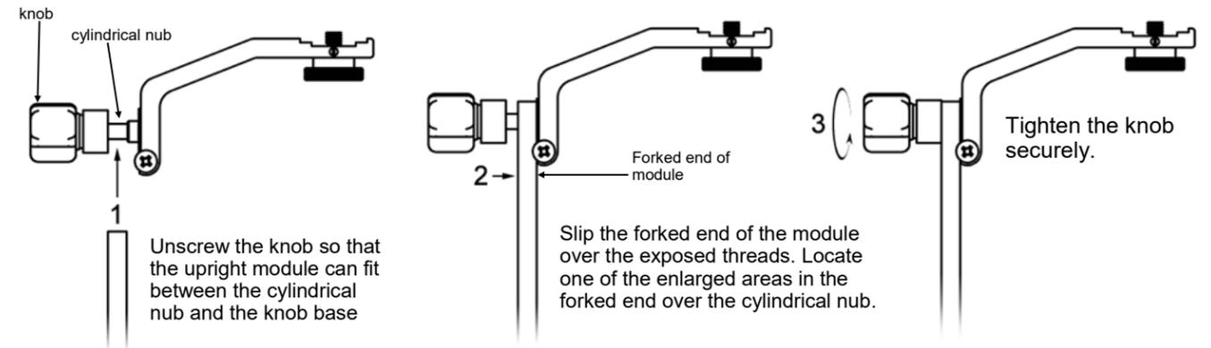
Unscrew the knob so that the upright module can fit between the cylindrical nub and the knob base
