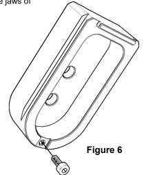
**Safety Stop Channels** We recommend using clamps with safety stop channels. These channels allow a full range of forward and back motion but will not let the block slip out if the clamp is inadvertently loosened.
