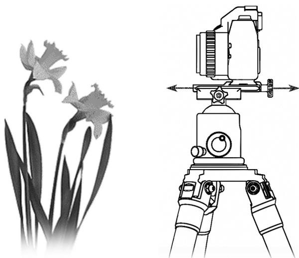
**Caution:** When using the perpendicular plate as a macro slider, you may end up sliding the plate so far back in the clamp that it is no longer properly clamped.
