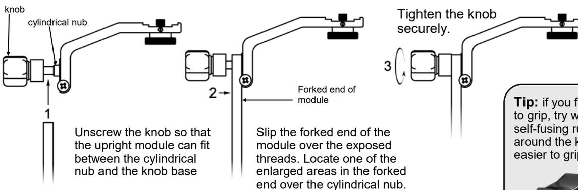
**Tip:** if you find the metal knobs difficult to grip, try wrapping several layers of self-fusing rubber grip tape (**3M 2155**) around the knob to cushion it and make it easier to grip in the field.
