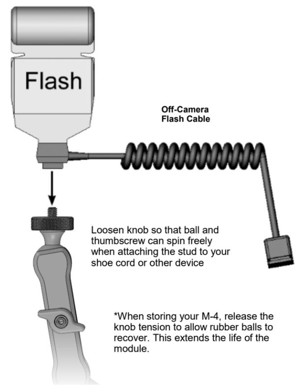
\*When storing your M-4, release the knob tension to allow rubber balls to recover. This extends the life of the module.
