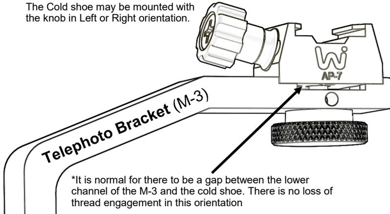
\*It is normal for there to be a gap between the lower channel of the M-3 and the cold shoe. There is no loss of thread engagement in this orientation
