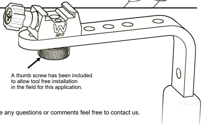
A thumb screw has been included to allow tool free installation in the field for this application.
