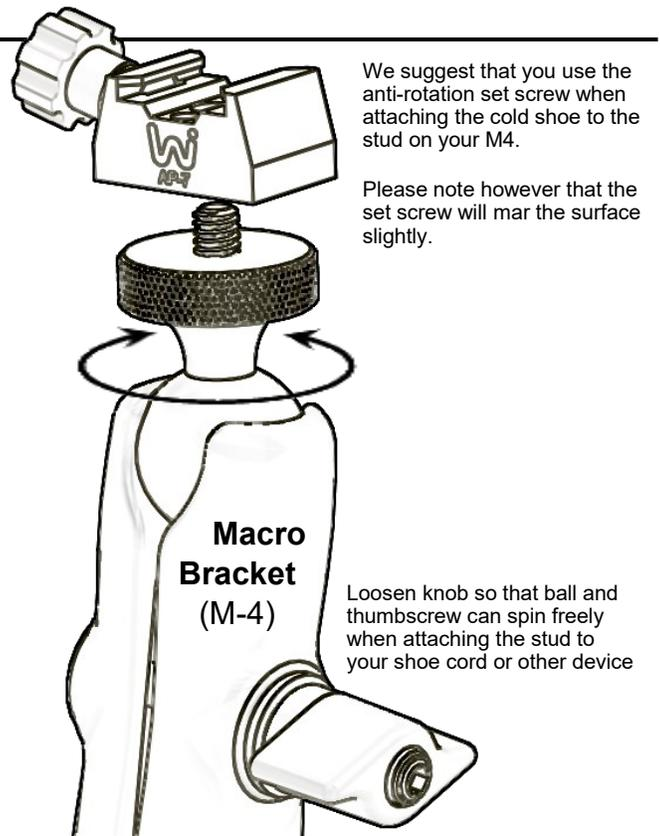
We suggest that you use the anti-rotation set screw when attaching the cold shoe to the stud on your M4.
