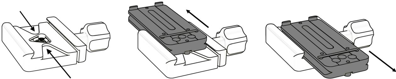
**⚠️ 3rd Party Clamp Warning:** Our safety stop screws work with most 3rd party quick-release clamps, but clamps that do not have channels and are too wide to be straddled by the safety stop screws will not work.
