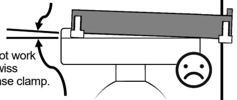
Clamps without safety stop channels (or those without adequate clearance) will **insecurely** clamp the block at an angle
